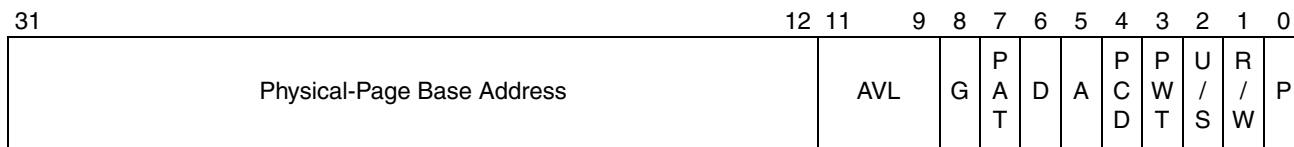
Figure 5-6. 4-Kbyte PTE—Non-PAE Paging Legacy-Mode
